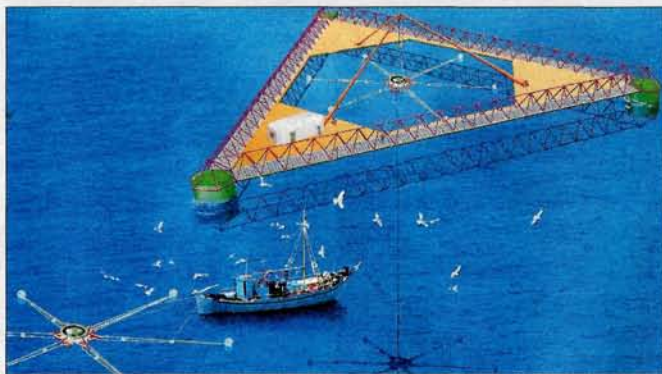
Artists's impression of the Delta Berenike ballasted floating platform being made for the NESTOR underwater detector. The 60 m triangular platform (hence Delta) is shown with an array of photodetectors. Berenike was the wife of Ptolemy III and Coma Berenikes is a galaxy in the Bootes constellation.
