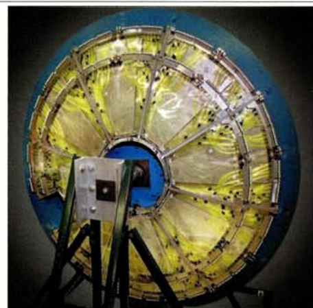
The Forward Preshower Detector (FPS) built at Brookhaven.
