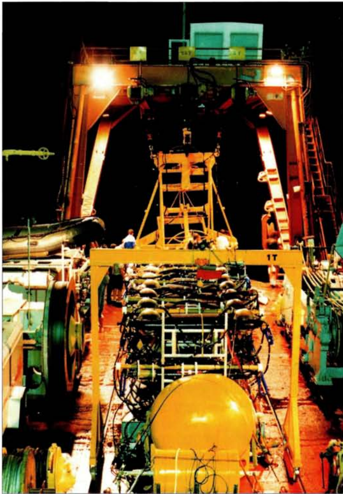
A prototype ANTARES detector line safely back on board after underwater tests.
