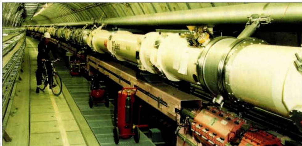
The HERA electron-proton collider at DESY, showing the superconducting proton ring (top) and the electron ring (below). The major components were designed and built in other countries.
